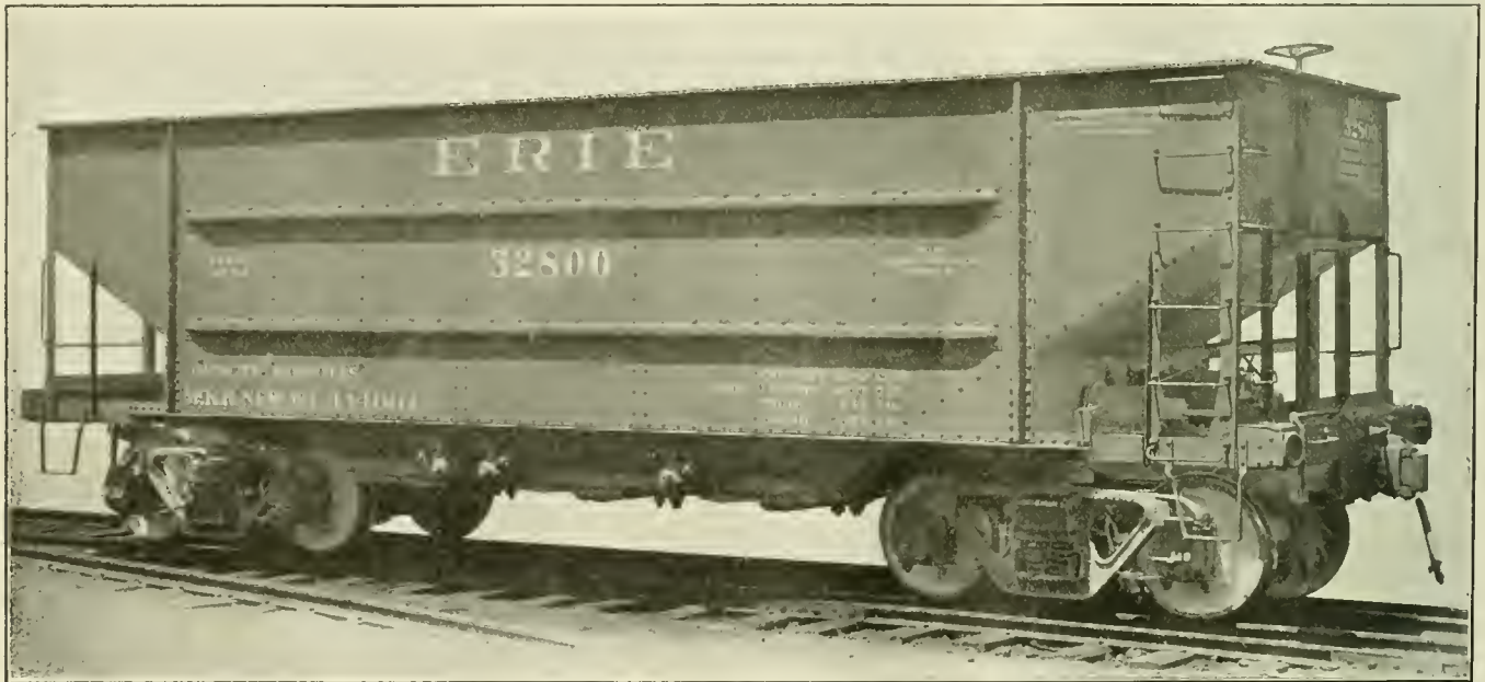
TYPE OF SELF-CLEARING TRIPLE HOPPER BOTTOM CARS FOR THE ERIE RAILROAD. PRESSED STEEL CAR COMPANY, BUILDERS.
